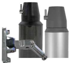
Perfect for boat 50 to 70 feet, this unique "socket" type mast end fitting automatically locks onto the TS style mast toggle pin with a quick and easy push. The release is just as quick with a press of the lever. Universal socket design fits either the T-125 or T-150 size mast connection
